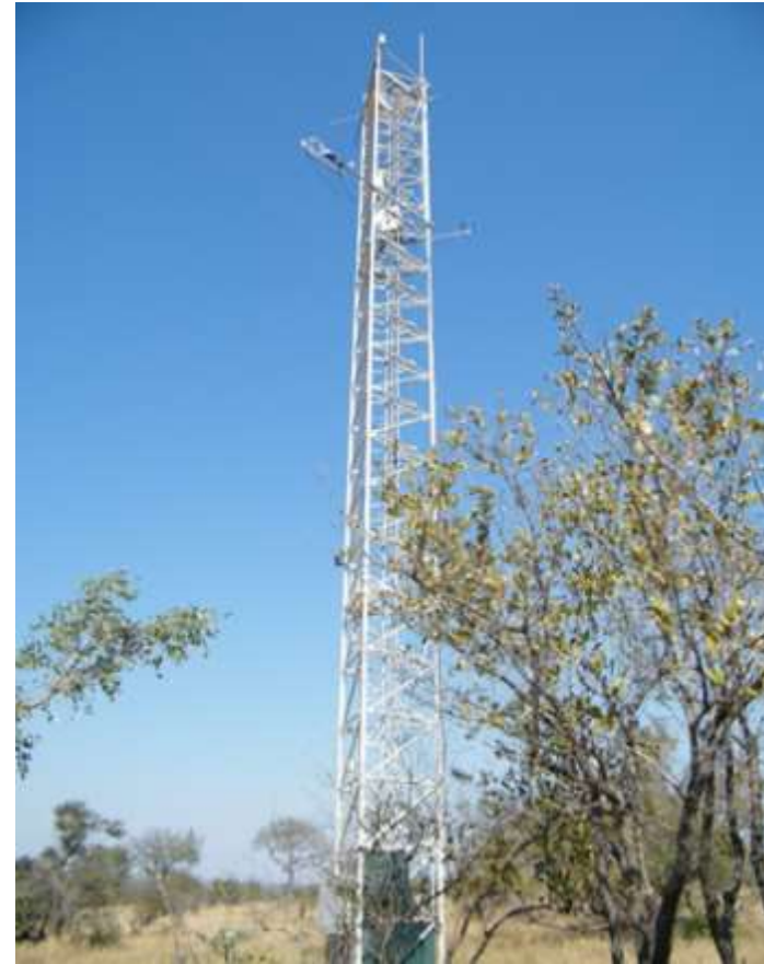
Eddy-covariance flux tower at Skukuza. An example of sophisticated research infrastructure for ecology
